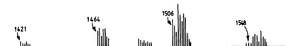
Fig. 4 Field desorption mass spectrum of the product of short acetylation of bleomycin A_2 ; demethylated cationised molecular ions are present at m/z 1464, 1467 (1:1, mono-acetyl), 1506, 1509, 1512 (1:2:1, di-acetyl) and 1548, 1551, 1554, 1557 (1:3:3:1, tri-acetyl).
